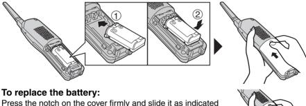
Press the notch on the cover firmly and slide it as indicated by the arrow. Replace the old battery with a new one (p. 9). Close the cover and charge the battery for about 6 hours.
